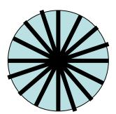
• Then straight across the spoke pattern, apply strips in one direction overlapping half the width of the tape. When you have completed, apply tape the other direction again overlapping half the width of the tape resulting in a grid pattern.
