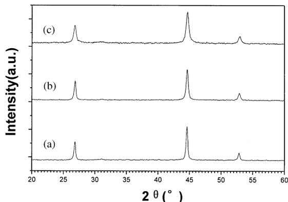
Fig. 3. Powdered XRD patterns of  $\text{Cu}_{2-x}\text{Se}$  prepared in the presence of different complexing agents: (a) TSC; (b) TEA; and (c) without any complexing agent.
