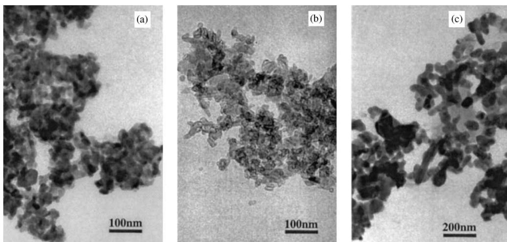
Fig. 2. TEM images of copper selenides: (a)  $\text{Cu}_{2-x}\text{Se}$ ; (b)  $\text{Cu}_3\text{Se}_2$ ; and (c)  $\text{CuSe}$ .
