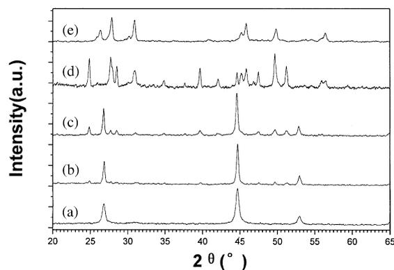
Fig. 1. Powdered XRD patterns of copper selenides: (a)  $\text{Cu}_{2-x}\text{Se}$ ; (b,c) mix-phased  $\text{Cu}_{2-x}\text{Se}$  and  $\text{Cu}_3\text{Se}_2$ ; (d)  $\text{Cu}_3\text{Se}_2$ ; and (e)  $\text{CuSe}$ .
