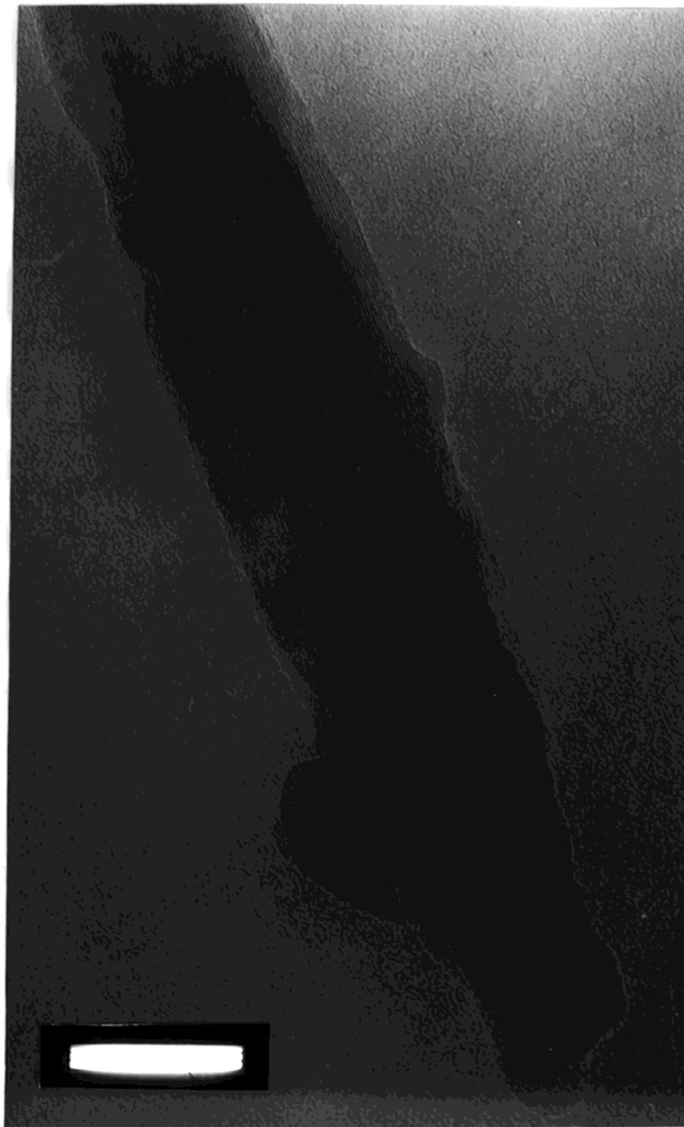
**Figure 3.** HRTEM image of the as-prepared  $\text{Bi}_2\text{S}_3$  nanorods (bar = 20 nm).
