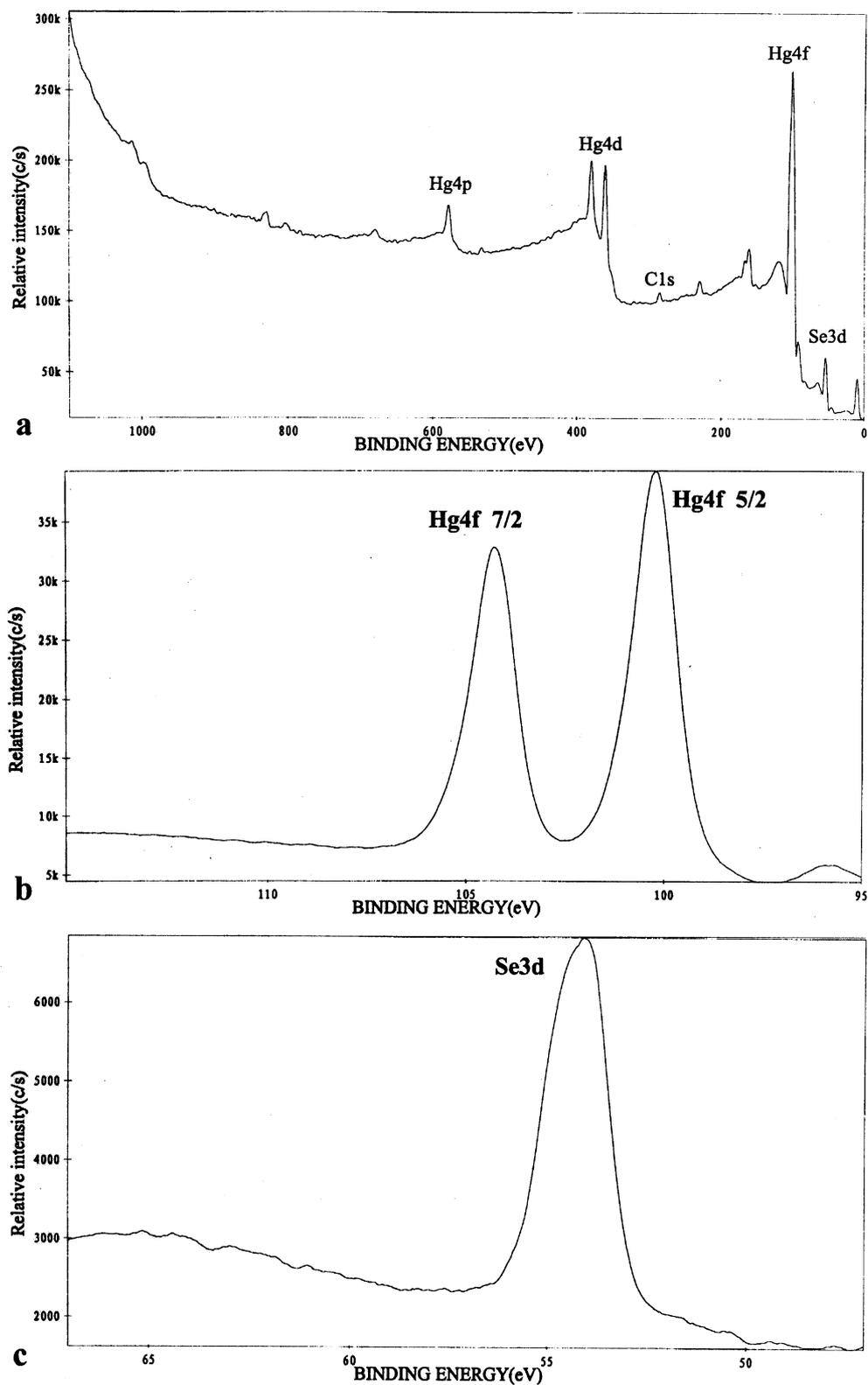
Fig. 4. (a) Wide XPS picture of HgSe nanoparticles; high-resolution XPS picture; (b) Hg4f; (c) Se3d.
