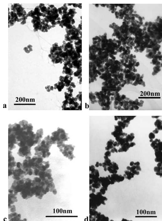
Fig. 3. TEM images of HgSe nanoparticles prepared in the presence of different complexing agents: (a) ethylenediamine; (b)  $\text{NH}_3$ ; (c) TEA ( $0.200 \text{ mol l}^{-1}$ ); (d) TEA ( $0.133 \text{ mol l}^{-1}$ ).
