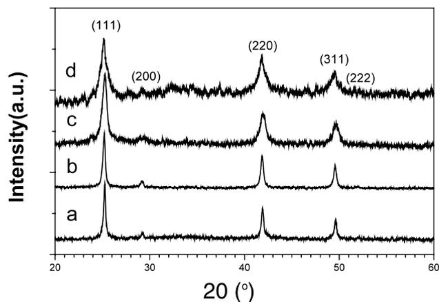
Fig. 1. XRD patterns of HgSe nanoparticles using different complexing agents: (a) without any complexing agent; (b) en; (c) NH<sub>3</sub>; (d) TEA (0.2 mol l<sup>-1</sup>).
