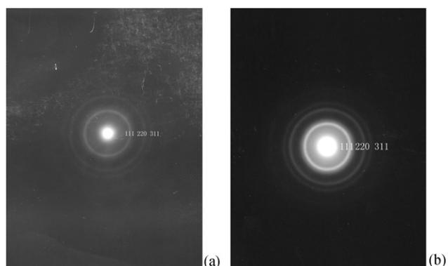
**Fig. 4** SAED images of CeO<sub>2</sub> nanoparticles (a) prepared by microwave irradiation; (b) prepared by ultrasonic irradiation.
