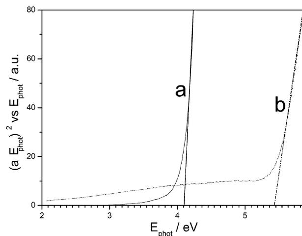
**Fig. 8** Plots of  $(\alpha E_{\text{phot}})^2$  vs.  $E_{\text{phot}}$  for direct transitions of CeO<sub>2</sub> nanoparticles (a) prepared by microwave irradiation; (b) prepared by ultrasonic irradiation.
