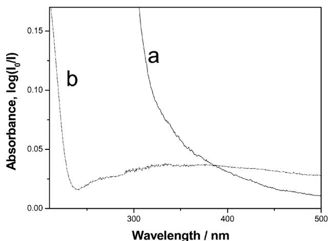
**Fig. 7** The UV-Vis absorbance spectra of CeO<sub>2</sub> nanoparticles (a) prepared by microwave irradiation; (b) prepared by ultrasonic irradiation (in ethanol suspension).
