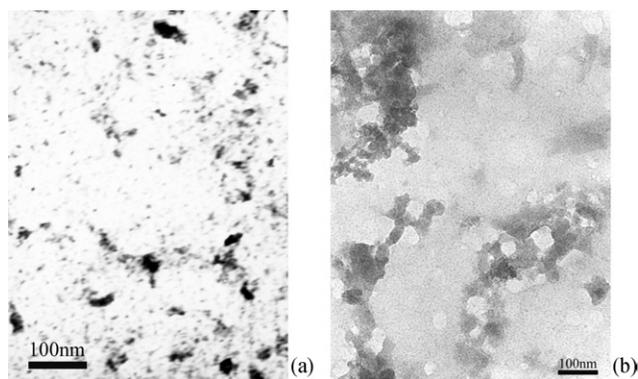
**Fig. 3** TEM images of CeO<sub>2</sub> nanoparticles (a) prepared by microwave irradiation; (b) prepared by ultrasonic irradiation.
