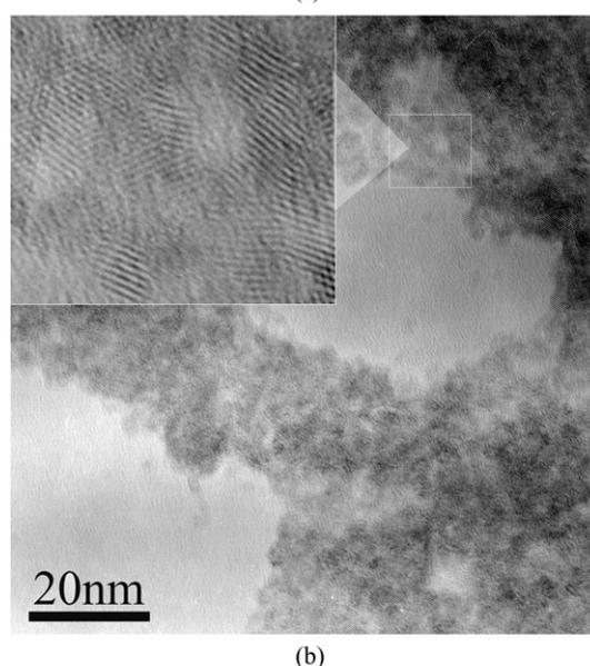
**Fig. 5** HRTEM images of CeO<sub>2</sub> nanoparticles (a) prepared by microwave irradiation; (b) prepared by ultrasonic irradiation.
