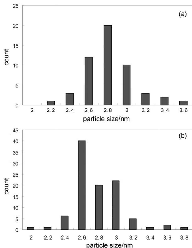
**Fig. 6** The particle size distribution picture measured directly from HRTEM: (a) CeO<sub>2</sub> nanoparticles prepared by microwave heating method; (b) CeO<sub>2</sub> nanoparticles prepared by sonochemical method.
