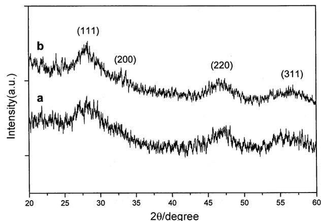
**Fig. 1** Powder XRD patterns of  $\text{CeO}_2$  nanoparticles (a) prepared by microwave irradiation; (b) prepared by ultrasonic irradiation.
