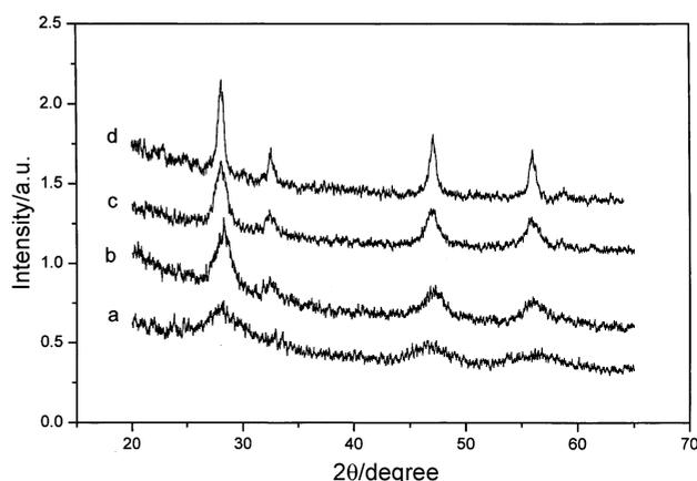
**Fig. 2** Powder XRD patterns of  $\text{CeO}_2$  nanoparticles prepared sonochemically sintered at different temperatures: (a) as-prepared; (b) sintered at  $300^\circ\text{C}$  for 2 h; (c) sintered at  $500^\circ\text{C}$  for 2 h; (d) sintered at  $700^\circ\text{C}$  for 2 h.
