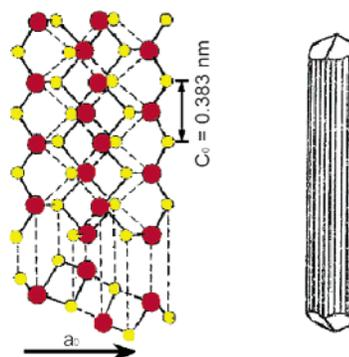
**Figure 6.** Schematic illustration of the structure of an  $\text{Sb}_2\text{S}_3$  nanorod. The red spheres represent the S atoms, and the yellow spheres represent the Sb atoms. It is viewed along the (010) direction. The nanorod grows along the (001) crystal face.
