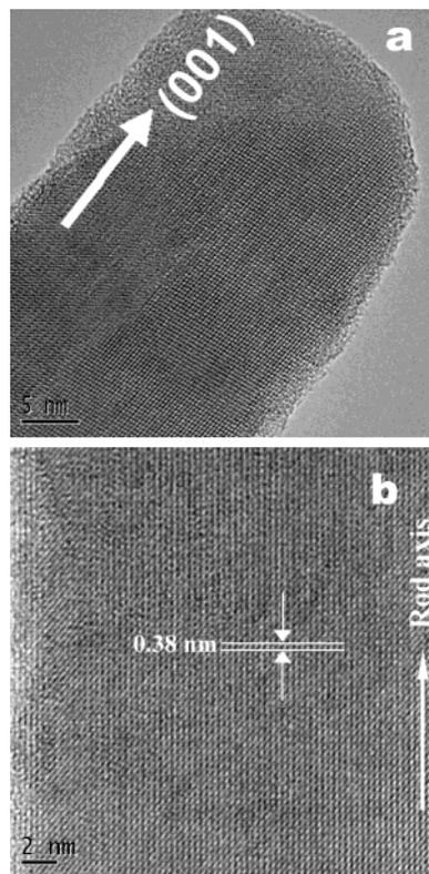
**Figure 5.** (a) HRTEM image of an individual  $\text{Sb}_2\text{S}_3$  nanorod. (b) HRTEM image with a higher magnification, revealing the microstructure inside an  $\text{Sb}_2\text{S}_3$  nanorod.
