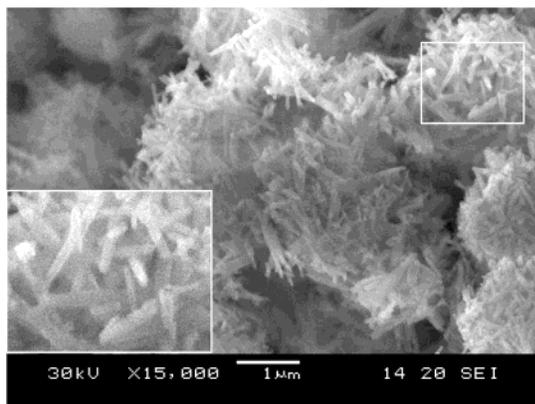
**Figure 3.** Typical SEM image of the as-prepared  $\text{Sb}_2\text{S}_3$  nanorods.
