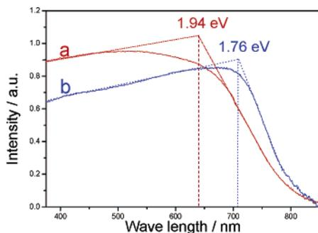
**Figure 7.** Diffuse reflection spectra of (a) the as-prepared  $\text{Sb}_2\text{S}_3$  nanorods and (b) rodlike  $\text{Sb}_2\text{S}_3$  bulk crystals (with average diameter of  $1.5 \mu\text{m}$  and length of  $20 \mu\text{m}$ ).
