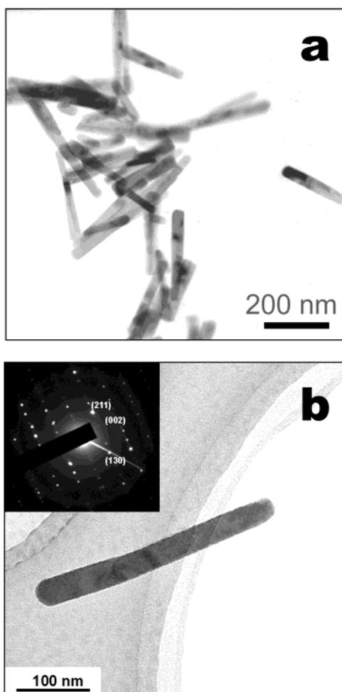
**Figure 4.** (a) Typical TEM image of the as-prepared  $\text{Sb}_2\text{S}_3$  nanorods. (b) TEM image of an individual  $\text{Sb}_2\text{S}_3$  nanorod. The inset is the SAED pattern recorded on this rod.
