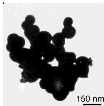
**Figure 4.** TEM image of  $\text{Sb}_2\text{S}_3$  powders prepared by refluxing the reactant mixture by means of conventional heating for 2 h. The powder XRD measurement shows that this sample is orthorhombic  $\text{Sb}_2\text{S}_3$ . The EDAX result shows that the Sb/S atomic ratio of this sample is 1:1.45.
