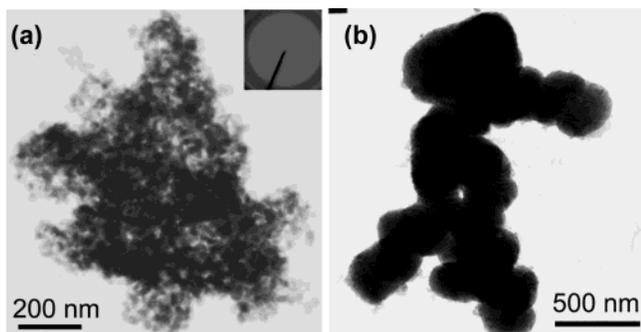
**Figure 5.** (a) TEM image of  $\text{Sb}_2\text{S}_3$  powders prepared by choosing ethanol as the solvent. The inset is the corresponding SAED pattern. The Sb:S ratio of this sample is calculated to be 1:1.40 according to the EDAX results. (b) TEM image of  $\text{Sb}_2\text{S}_3$  powders prepared by using triethylene glycol as the solvent. Powder XRD measurement shows that this sample is orthorhombic  $\text{Sb}_2\text{S}_3$ . The EDAX result shows that the Sb/S ratio is 1:1.48.
