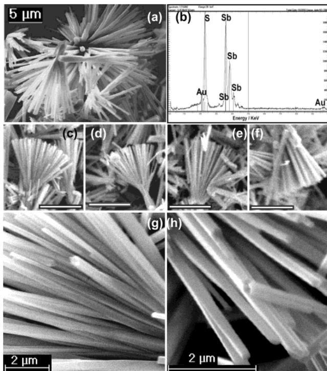
**Figure 1.** (a) Typical SEM image with low magnification revealing the overall morphology of several bunches of radial arrays composed of whiskers. (b) EDAX pattern of the  $\text{Sb}_2\text{S}_3$  whiskers shown in Figure 1a. (c–f) Several SEM images showing individual bunches of radial arrays. The length of the bars equals  $10\ \mu\text{m}$ . (g and h) SEM images with higher magnifications showing sectional images of radial arrays.
