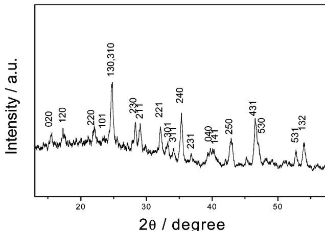
**Figure 2.** XRD pattern of the as-prepared  $\text{Sb}_2\text{S}_3$  powders.
