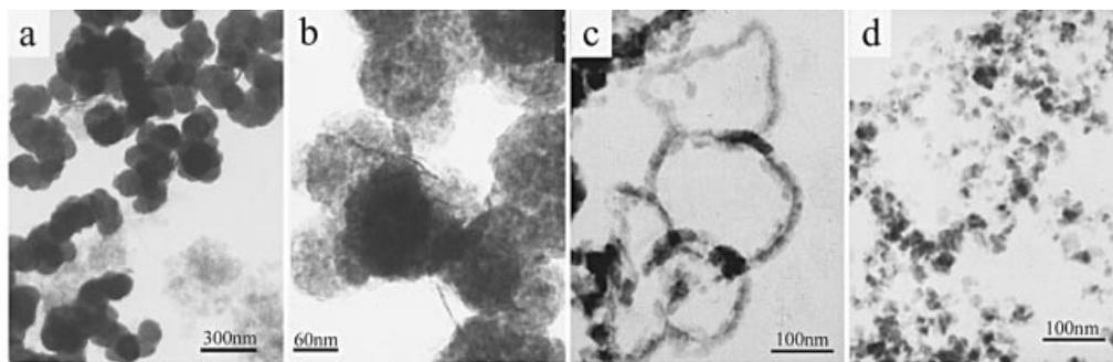
Figure 7. TEM images of the CdS particles obtained with different thiourea/thioacetamide ratios as the sulfur source (sonic intensity: 20 W/cm<sup>2</sup>; sonication time: 30 min): (a) thioacetamide as the sulfur source; (b) with a 1:1 ratio of thiourea/thioacetamide; (c) with a 4:1 ratio of thiourea/thioacetamide; (d) thiourea as the sulfur source
