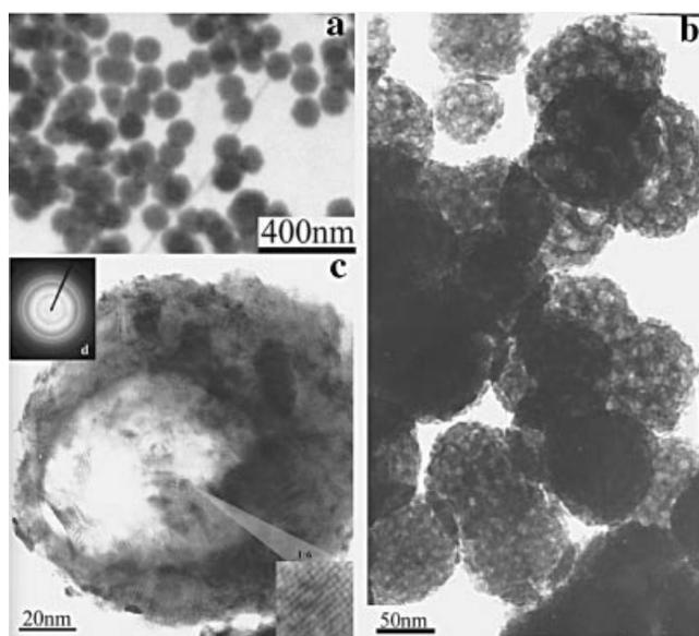
Figure 2. TEM and HRTEM images of the CdSe assemblies in the presence of ammonia after sonication for 30 min (concentration of  $\text{NH}_3$ : 0.8 mol/L): (a, b) TEM images of the product, (c) HRTEM image of an individual CdSe hollow-spherical assembly, (d) [inset in (c)] SAED pattern recorded on the hollow sphere shown in (c)
