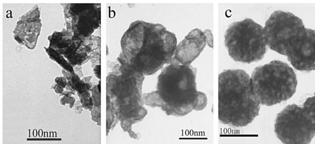
Figure 5. TEM images of the products at different stages of fabricating CdSe hollow spheres (sonic intensity is  $20 \text{ W/cm}^2$ ): (a) cadmium hydroxide particles at the initial stage (immediately after precipitation); (b) after 15 min reaction; (c) after 30 min reaction
