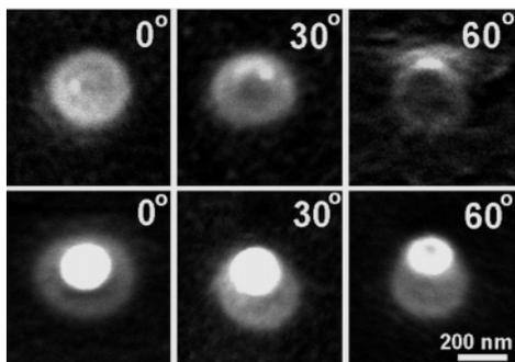
**Figure 4.** SEM images of (top) a nanoshell partially embedded in PDMS and (bottom) a nanoshell heterodimer consisting of two nanoshells with different core and shell dimensions. The images were taken using tilt = 0°, 30°, and 60°.
