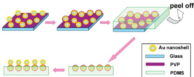
**Figure 1.** Schematic illustration of the fabrication of nanoshell dimers.
