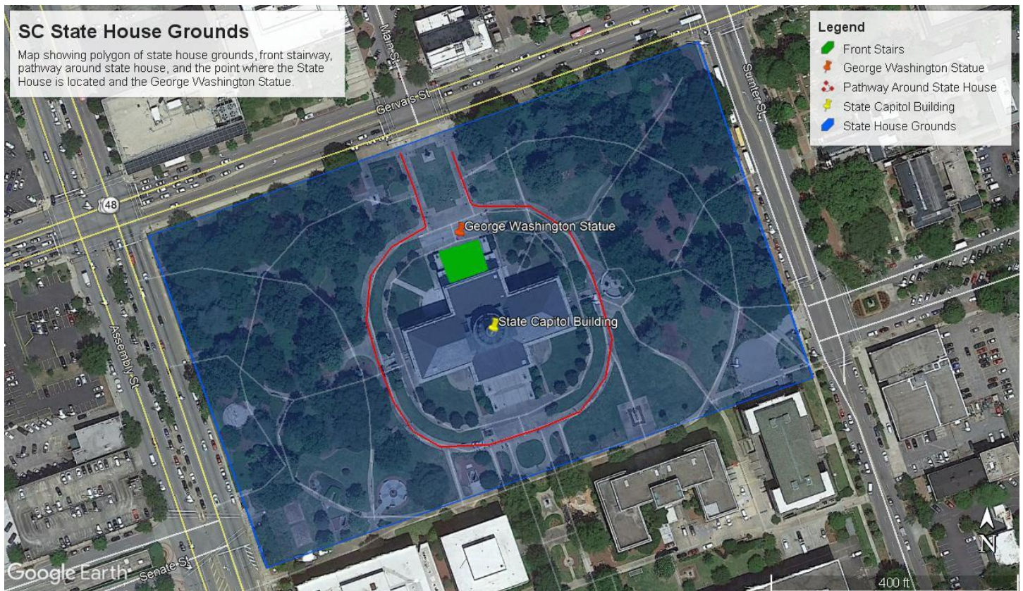
Figure 2 This is an illustration of how you can map points, lines, and polygons of different structures, features, and areas with various colors and labels to illustrate the size and characteristics of your site over aerial imagery.
